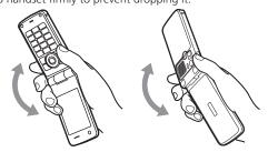
**3** Pat handset with a dry cloth to remove any water remaining in microphone, earpiece, speaker, keypad, hinge, etc.
