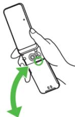
**3 Pat handset against a clean dry cloth to remove remaining water from Microphone, Earpiece, Speaker, keypad, hinge, etc.**
