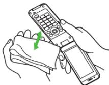
**4 Remove Battery Cover, and wipe water drops off Inner Cover area and Battery Cover underside. Replace Battery Cover.**
