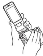
**2 Hold handset firmly. Shake handset about 20 times until no water drops come out. Repeat on all sides.**
