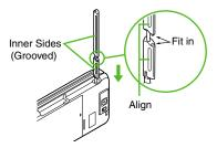
Retract Antenna, aligning top and bottom parts, inner sides down; fold it down then push it in until bead fits snugly into dimple.
